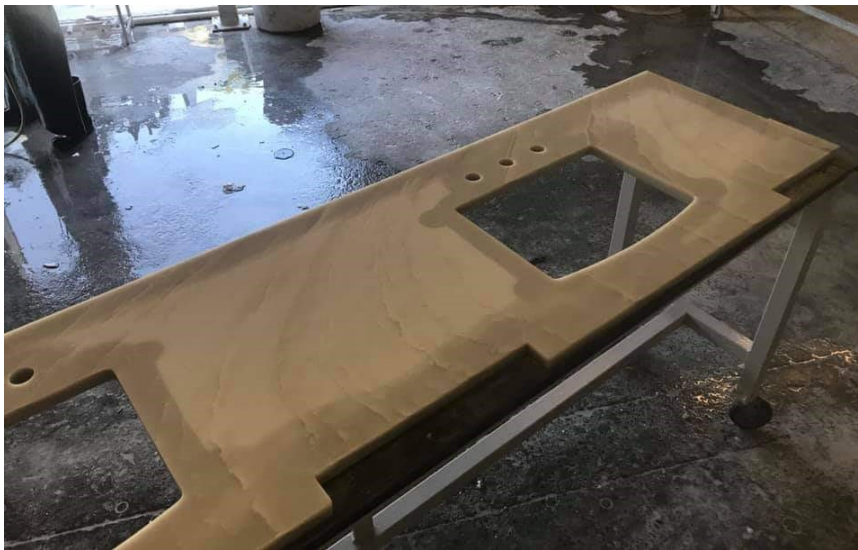
Fig. 1: Edge staining caused by absorption of moisture after water jet cutting
